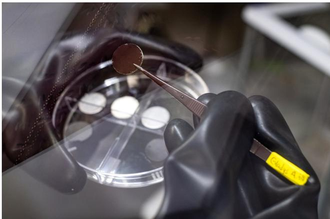
Rice University graduate student Gladys López-Silva holds a lithium metal anode with a film of carbon nanotubes. Once the film is attached, it becomes infiltrated by lithium ions and turns red. Credit: Jeff Fitlow/Rice University
