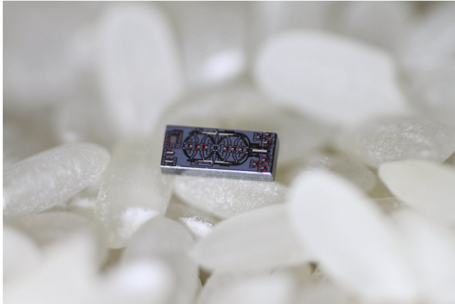
The optical gyroscope developed in Ali Hajimiri's lab, resting on grains of rice. Credit: Ali Hajimiri/Caltech
