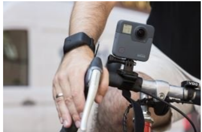
Physical stress reactions are measured by the smart band sensor. At the same time, the video camera records the surroundings. Credit: Patrick Langer, KIT
