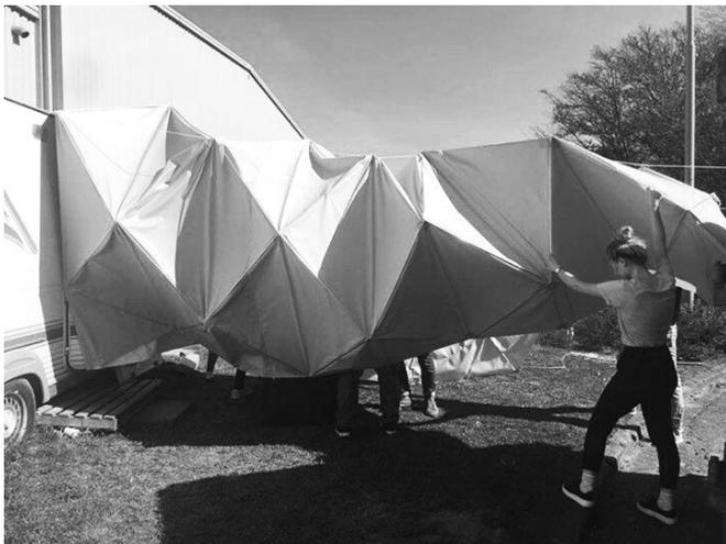
The prototype was deployed and tested to extreme conditions on the 20th of April during the EuroMoonMars2018 simulation at ESA – ESTEC. The origami structure was designed as a gateway and sub-system between the exo-habitat, airlock system and exo-laboratory. Credit: Anna Sitnikova
