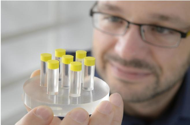
Adhesion to rough surfaces is significantly improved by the combination of two materials. The large-scale model shows the basic principle and the structure of the new adhesives, where soft materials (yellow) are applied to harder materials. Credit: Iris Maurer
