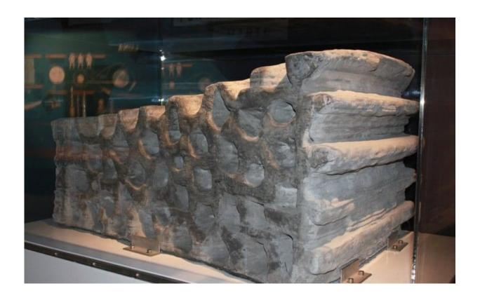
This 1.5 tonne building block was produced as a demonstration of 3D printing techniques using lunar soil. The design is based on a hollow closed-cell structure – reminiscent of bird bones – to give a good combination of strength and weight. Credit: ESA
