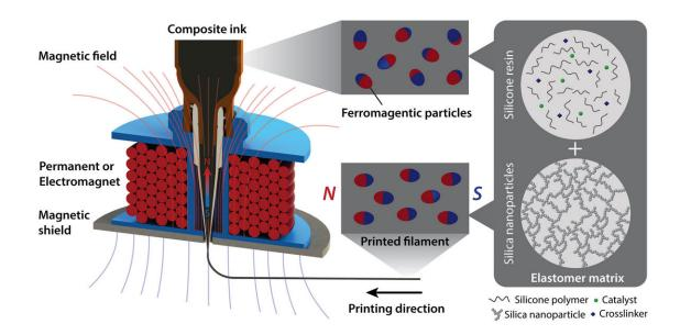
The schematics of the printing process and the material composition. The ferromagnetic particles embedded in the composite ink are reoriented by the applied magnetic field prior to printing. Credit: US Army
