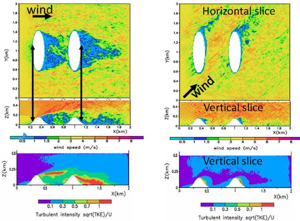
Fig.2 ABL-ABL model simulated fine scale turbulent flow over double ridges: Only wind direction changes (left panel: west wind; right panel: southwest wind) resulted very different mean flow and turbulence fields.
