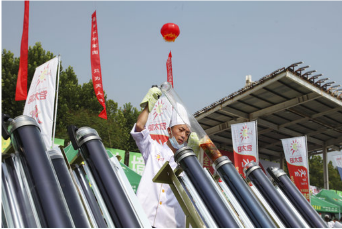
In this photo taken Thursday, Aug. 2, 2018, a chef prepares to cook food in a solar cooker which uses a metal and glass vacuum tube heated by mirrors curved to capture the sun's heat in Dezhou in the eastern Shandong province in China. Two dozen chefs with white aprons and hats cooked soups, baked buns, potatoes, and boiled rice at a festival to demonstrate the potential of solar cookers that organizers claim can help reduce climate-changing greenhouse gas emissions. (AP Photo/Fu Ting)
