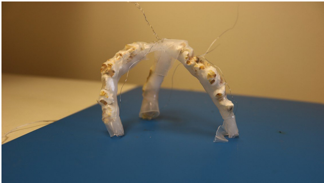
A soft robotic device powered by popcorn, constructed by researchers in Cornell's Collective Embodied Intelligence Lab. Credit: Cornell University
