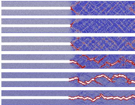
Measuring fracture energy in model glasses with various ductility; showing the deformation morphologies for glasses with various ductilities; and measured fracture energy (and normalized fracture energy by the surface energy). Credit: Binghui Deng and Yunfeng Shi
