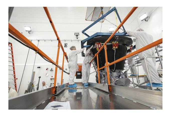
arker Solar Probe's heat shield, called the Thermal Protection System, is lifted and realigned with the spacecraft's truss as engineers from the Johns Hopkins Applied Physics Lab prepare to install the eight-foot-diameter heat shield on June 27, 2018. Credit: NASA/Johns Hopkins APL/Ed Whitman
