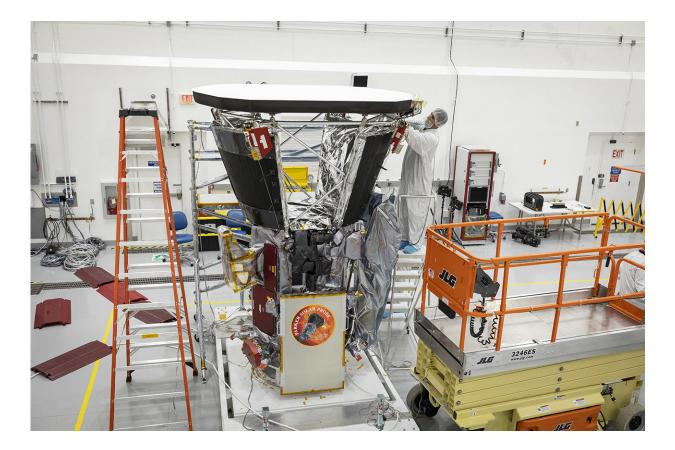
The Thermal Protection System connects to the custom-welded truss on the Parker Solar Probe spacecraft at six points to minimize heat conduction. Credit: NASA/Johns Hopkins APL/Ed Whitman
