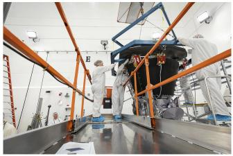
the spacecraft. At Parker Solar Probe's closest approach to the Sun, temperatures on the heat shield will reach nearly 2,500 degrees Fahrenheit, but the spacecraft and its instruments will be kept at a relatively comfortable temperature of about 85 degrees Fahrenheit.
