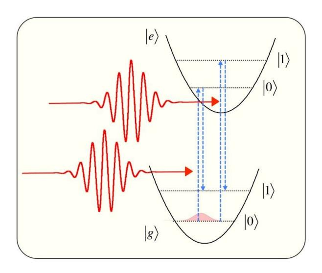
Coherent optical phonons are coherently controlled by a pair of ultrashort optical pulses. lg> and le> indicate the electronic ground and excited states and l0> and l1> indicate zero- and one-phonon state, respectively. Credit: Kazutaka G. Nakamura
