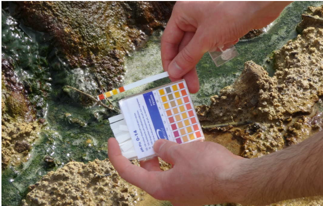
Measuring the pH of the water in the Dorset stream. Credit: Imperial College London
