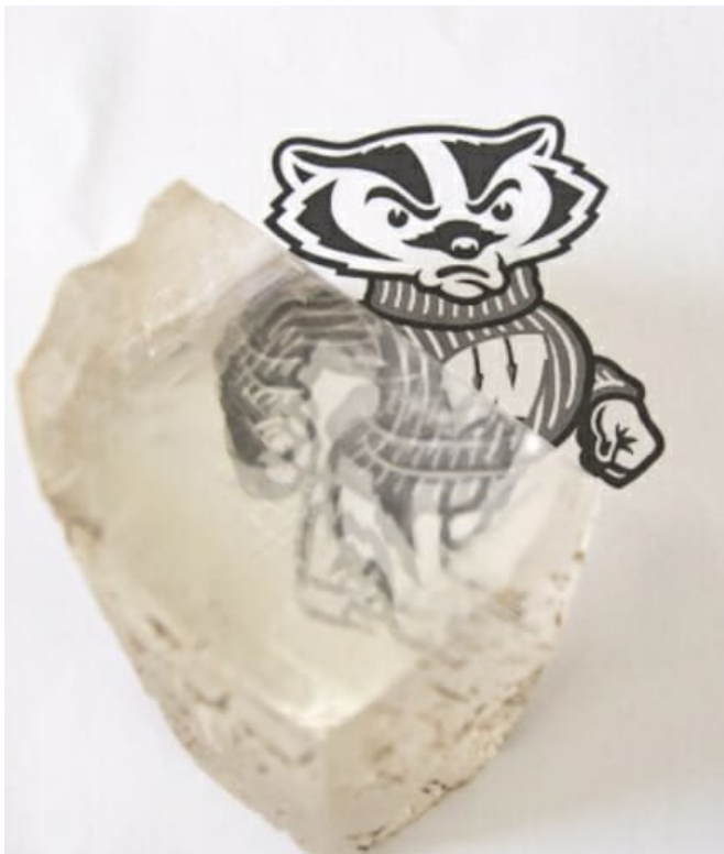
Calcite splits light due to a property called birefringence, causing a double image. Credit: Sam Million-Weaver
