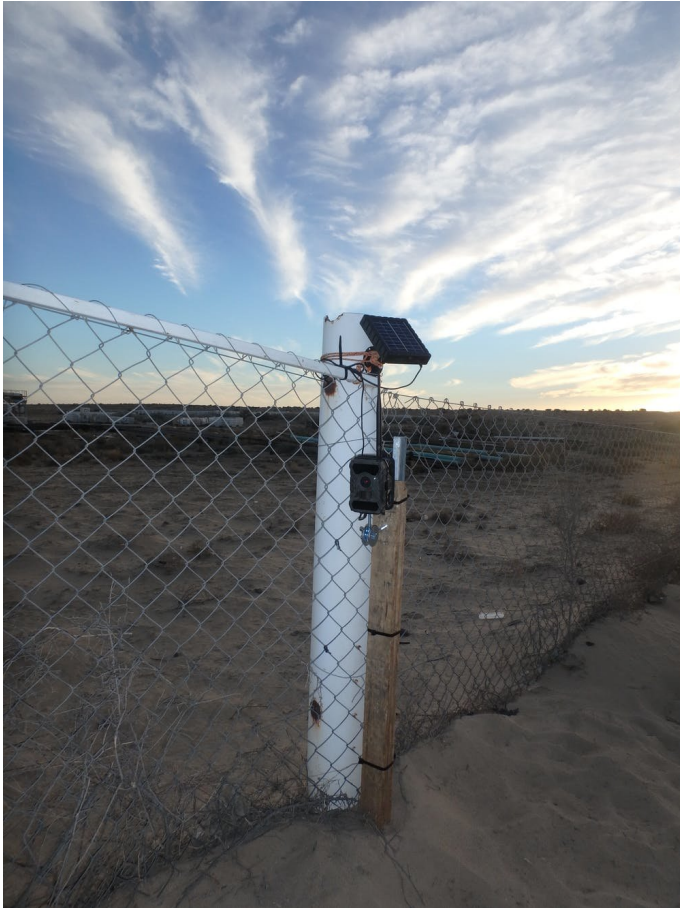
A 3G camera trap set in the Strzelecki Desert and sending images to the authors email and phone. Credit: PM, Author provided
