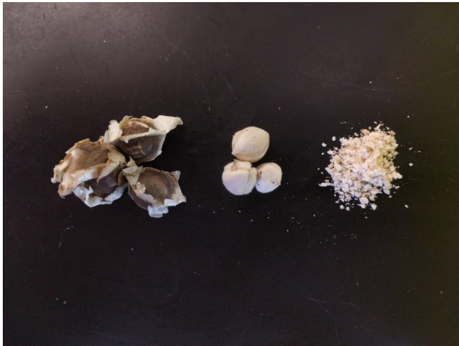
(left) Unshelled M. oleifera seeds, (middle) shelled seeds, (right) crushed seeds before protein extraction Credit: Carnegie Mellon University College of Engineering
