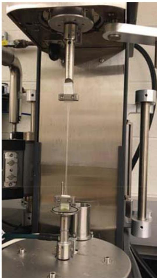
The adhesive strength of the material is tested in the lab.
