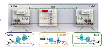
Illustration of the experimental setup for demonstrating ternary correlations. Credit: Hu et al. ©2018 American Physical Society
