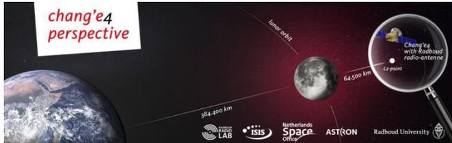
Behind the Moon the satellite revolves around a fixed point, the so-called second Lagrange point or L2 point of the Earth-Moon system. That point is about 65,000 kilometers from the Moon. Credit: Radboud Radio Lab?
