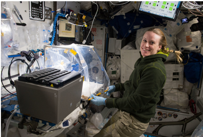
Astronaut Kate Rubins working with Wet Lab-2, a tool for quantitative gene expression analysis set for further testing this year. Credit: NASA
