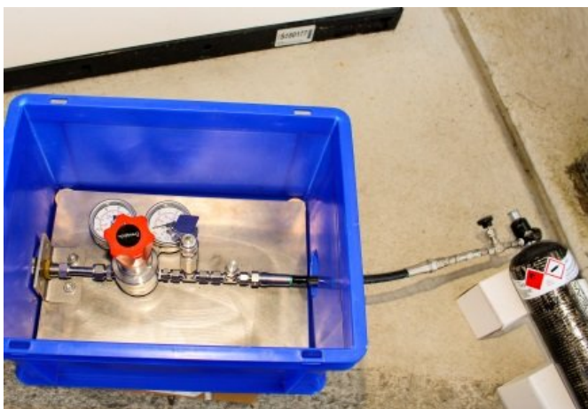
A successful project: The prototype connects the filling station with the gas bottle. Credit: Swiss Federal Laboratories for Materials Science and Technology
