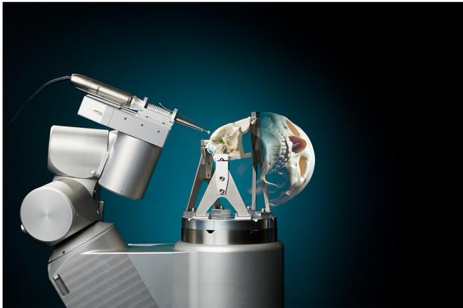
The robot of Jordan Bos with a phantom piece of skull base. The rest of the skull is added virtually to show where the piece is located in the body. Credit: Bart van Overbeeke
