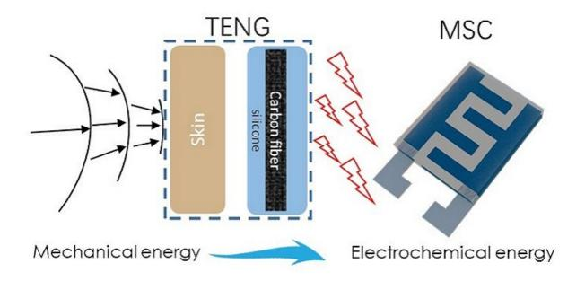
The wearable power bracelet can capture and transform energy from human motion into electricity and store it in MXene supercapacitors to drive different sensors. Credit: 2018 KAUST
