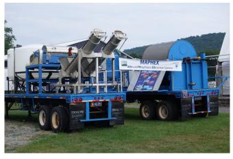
MAPHEX was designed to be a mobile system that fits on two large flatbed trailers to service a number of small-or medium-size dairies. If it is scaled up to have the capacity to treat manure from a large dairy, it would no longer be mobile. Credit: Hristov Research Group / Penn State
