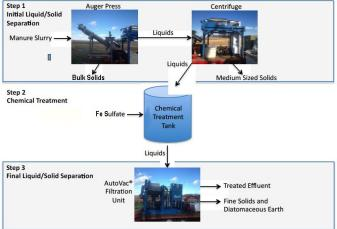
The system devised by Penn State and USDA scientists -- dubbed MAPHEX for MAnure PHosphorus Extraction -- involves a three-stage process, including liquid-solid separation with an auger press and centrifuge, chemical treatment with the addition of iron sulfate, and final filtration with diatomaceous earth. The machine is designed to process manure from manure-storage tanks or pits on dairy farms. Credit: Hristov Research Group/Penn State
