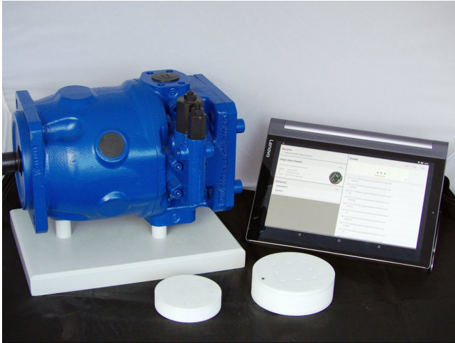
Demonstrator Hanover Trade Fair: configured wireless sensor nodes (in the foreground) send status messages of the axial piston pump (left) to a tablet. Credit: Fraunhofer IDMT
