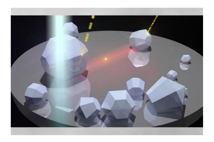
An electron beam (teal) hits a nanodiamond, exciting plasmons and vibrations in the nanodiamond that interact with the sample's nitrogen vacancy center defects. Correlated (yellow) photons are emitted from the nanodiamond, while uncorrelated (yellow) photons are emitted by a nearby diamond excited by surface plasmons (red). Credit: Raphael Pooser/Oak Ridge National Laboratory, US Department of Energy
