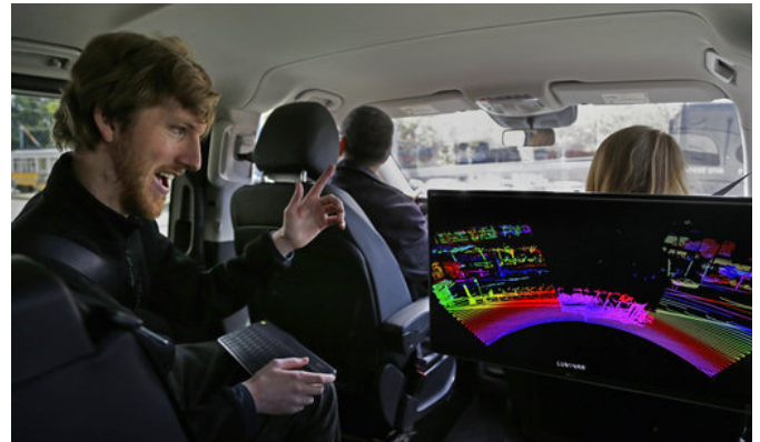
In this April 10, 2017, file photo, Luminar CEO Austin Russell gestures while looking at a 3D lidar map on a demonstration drive in San Francisco. Smaller versions of those spinning 360-degree mechanical laser sensors that sit atop self-driving cars are coming to mainstream vehicles. The lasers, called Lidar for Light Detection and Ranging, can see far-off objects in the dark, in bad weather, and in great detail. (AP Photo/Ben Margot, File)
