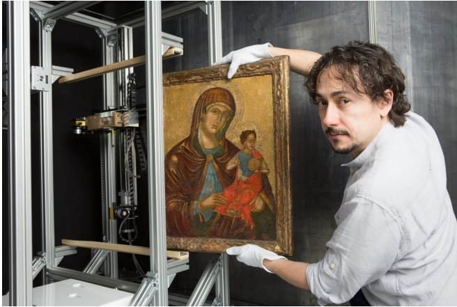
Slotting a painting into the X-ray scanner, which will analyse it at a high resolution. Credit: InsightArt s.r.o.
