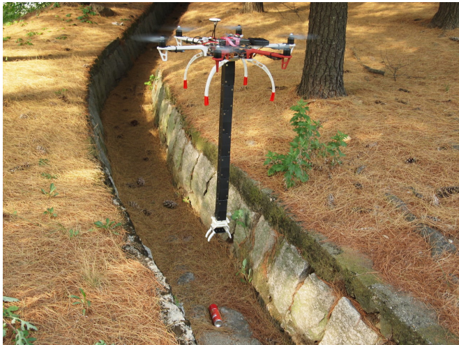
Drone with robotic arm can grip an object in the ditch. Credit: Seoul National University
