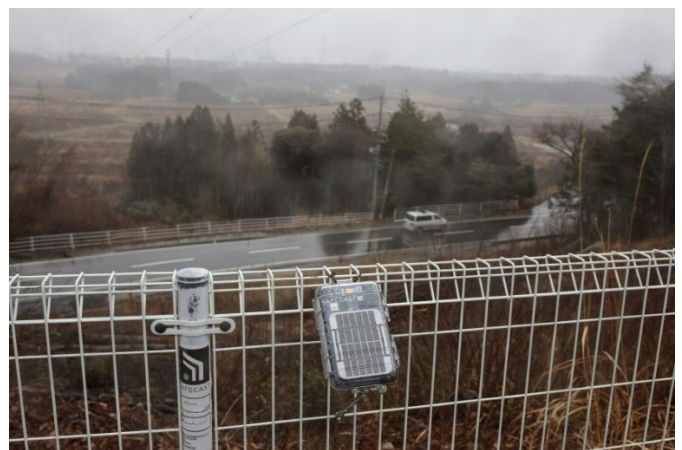
A geiger counter operated by the Safecast group is attached to a fence near the stricken Dai-ichi power plant
