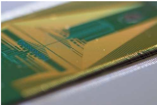
A large-scale integrated silicon-photonic quantum circuit for controlling multidimensional entanglement. Credit: University of Bristol
