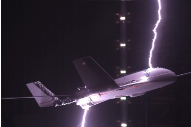
Lightning laboratory test on model aircraft. Credit: Joan Montanya/Polytechnic University of Catalonia
