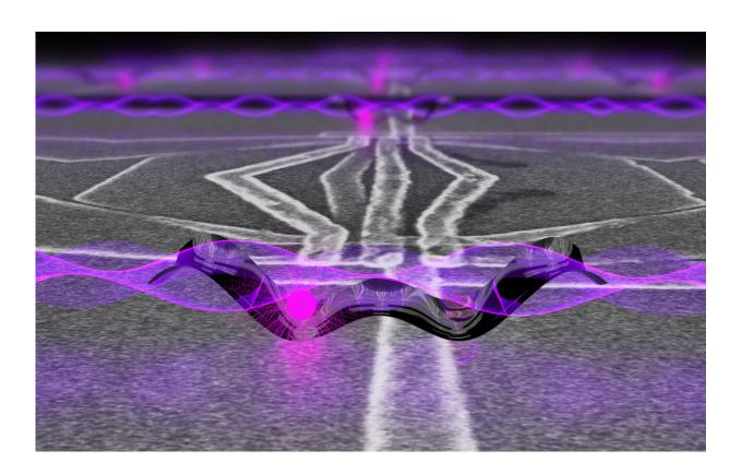
In a step forward for quantum computing in silicon -- the same material used in today's computers -- researchers successfully coupled a single electron's spin, represented by the dot on the left, to light, represented as a wave passing over the electron, which is trapped in a double-welled silicon chamber known as a quantum dot. The goal is to use light to carry quantum information to other locations on a futuristic quantum computing chip. Credit: Emily Edwards, University of Maryland.
