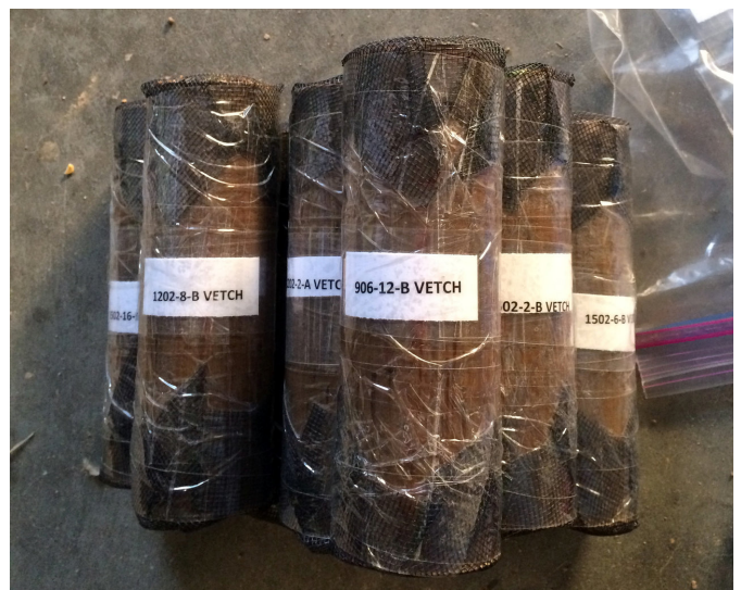
Soil cores with hairy vetch roots inside, ready to be buried in the field. After they are pulled back up, the soil will be washed off and the root biomass measured to look at rates of decomposition. Credit: Taylor Sievers.
