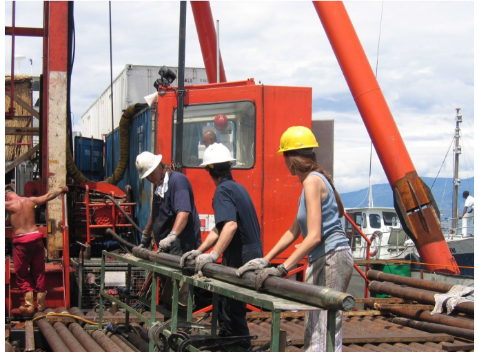
Members of the Lake Malawi Drilling Project science team handle the corer--part of the equipment used to collect sediment cores from the bottom Lake Malawi. Note the sediment in the end of the metal tube. Credit: the Lake Malawi Drilling Project
