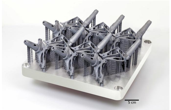
Several structural components arranged on a base plate after a selective laser melting process. Credit: Fraunhofer EMI
