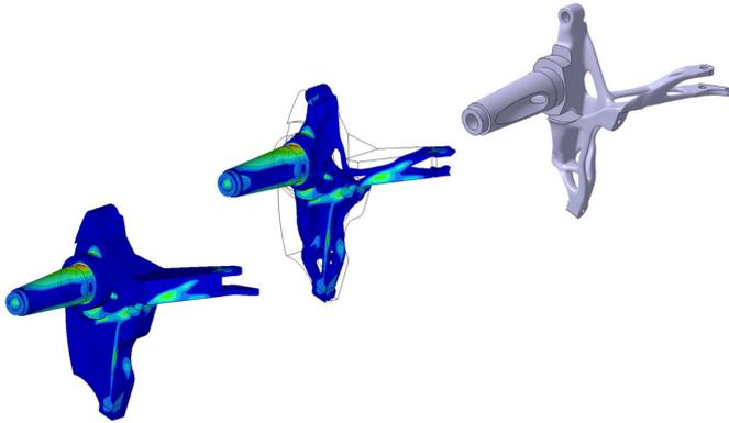
Finite element analysis of the start design of a wheel bearing technology demonstrator (left); numerical design optimization of the technology demonstrator to reduce the component's mass without impairing functionality (center); and CAD template for manufacturing the 3D metal component (right). Credit: Fraunhofer EMI
