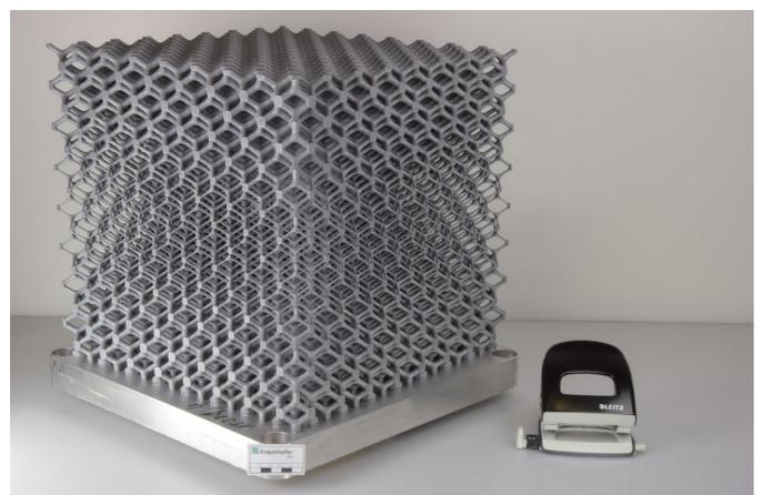
Lattice cube with edge length of 40 centimeters, one of the largest metal structures manufactured using selective
