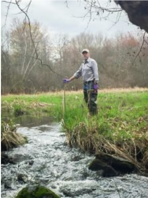
Professor John Clausen installing a stage sampler water collector device in the Conantville Brook. Credit: University of Connecticut
