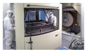
Together with their Virgo colleagues, the AEI researchers Harald Lück, Moritz Mehmet, and Henning Vahlbruch install the squeezed-light source, which was developed in Hannover, in a cleanroom at the Virgo gravitational-wave detector. Credit: H. Lück/B. Knispel/Max Planck Institute for Gravitational Physics
