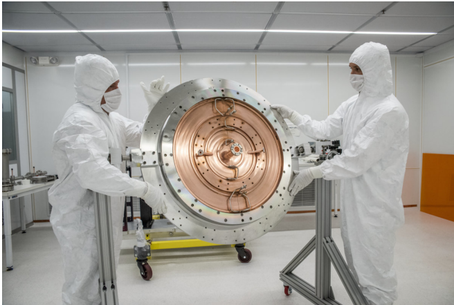
Joe Wallig, left, a mechanical engineering associate, and Brian Reynolds, a mechanical technician, work on the final assembly of the LCLS-II injector gun in a specially designed clean room at Berkeley Lab in August. Credit: Marilyn Chung/Berkeley Lab
