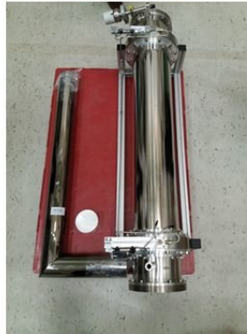
Standardized stainless-steel cylinder, which is used as a storage vessel and for measurements . Credit: Christopher Geppert, JGU Institute of Nuclear Chemistry
