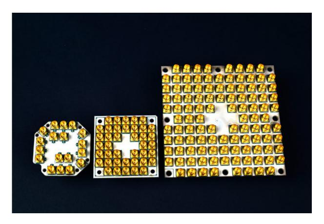
Intel Corporation is making fast progress scaling superconducting quantum computing test chips to higher qubit counts -- from 7, to 17 and now 49 qubits (left to right). Multiple gold connectors are required to control and operate each qubit. Credit: Walden Kirsch/Intel Corporation
