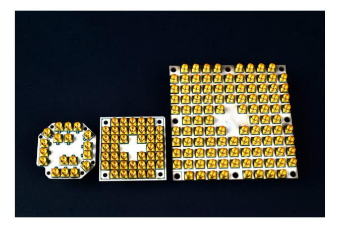
Intel Corporation is making fast progress scaling superconducting quantum computing test chips to higher qubit counts -- from 7, to 17 and now 49 qubits (left to right). Multiple gold connectors are required to control and operate each qubit. Credit: Walden Kirsch/Intel Corporation
