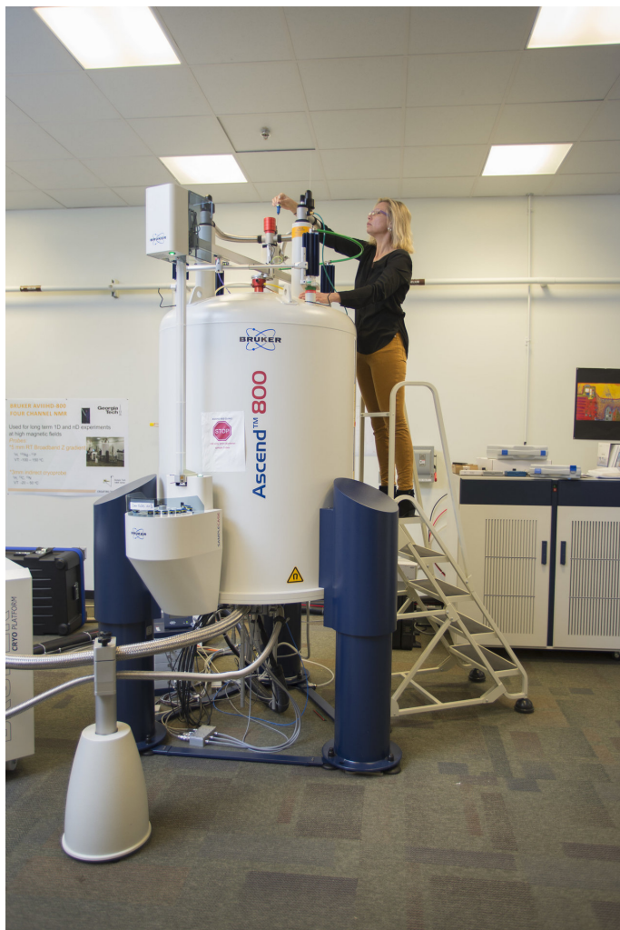
Principal investigator Julia Kubanek loads a sample into a nuclear magnetic resonance spectroscopy device. Credit: Georgia Tech / Christopher Moore
