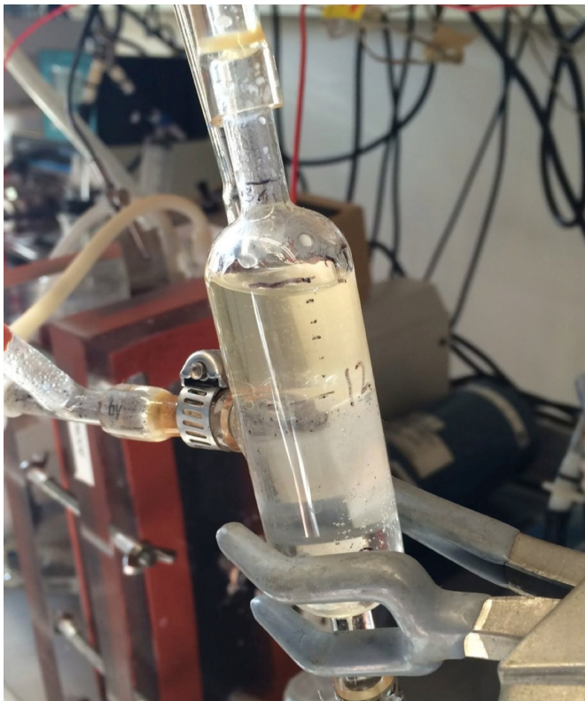
Photograph of bio-oil, made of caproic acid and caprylic acid, phase separates out at mildly acidic conditions. Credit: Lars Angenent, University of Tübingen
