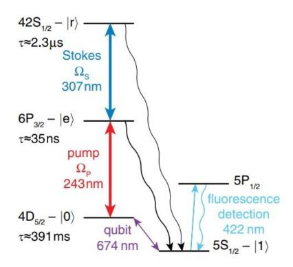
Using lasers, the researchers excited a strontium ion to the Rydberg state, which they then used to demonstrate a single-qubit Rydberg gate—one of the basic elements of the proposed trapped Rydberg ion quantum computer. Credit: Higgins et al. ©2017 American Physical Society
