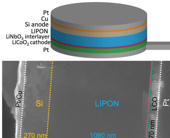
Schematic of full battery cell architecture and cross-sectional microscopic image of the actual battery. Credit: Sandia National Laboratories
