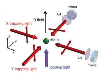
Rb atoms are trapped in a 2D lattice formed by two orthogonal retroreflected trapping beams at 1064 nm. The cooling light at 795 nm propagates along the magnetic field (z) and is sigma(–) -polarized. Credit: *Science* (2017). 10.1126/science.aan5614
