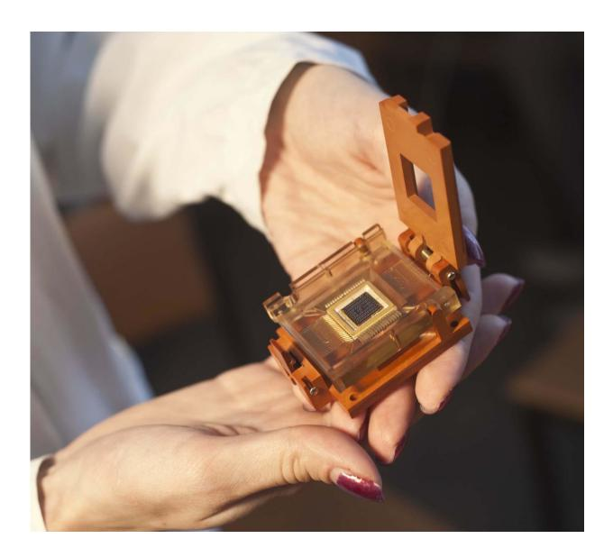
The memristive chip in its casing, housed in a standard contacting device (for testing the parameters of memristive nanostructures). Credit: Elena Emel'janova
