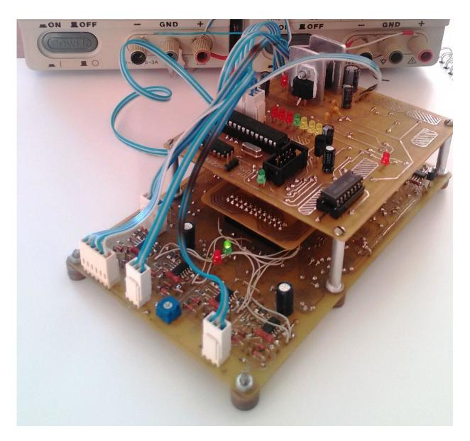
The prototype of an artificial neural network based on a hybrid analog-digital electronic circuit and a memristive chip. Credit: Elena Emel'janova
