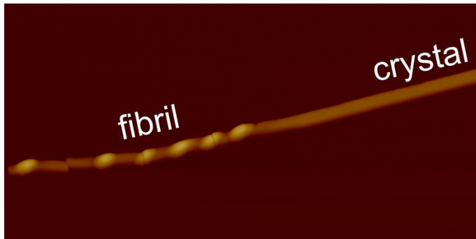
AFM 3-D Images of the peptides showing conversion from fibril (twisted) to crystals (untwisted). Credit: J. Adamcik/ETH Zurich
