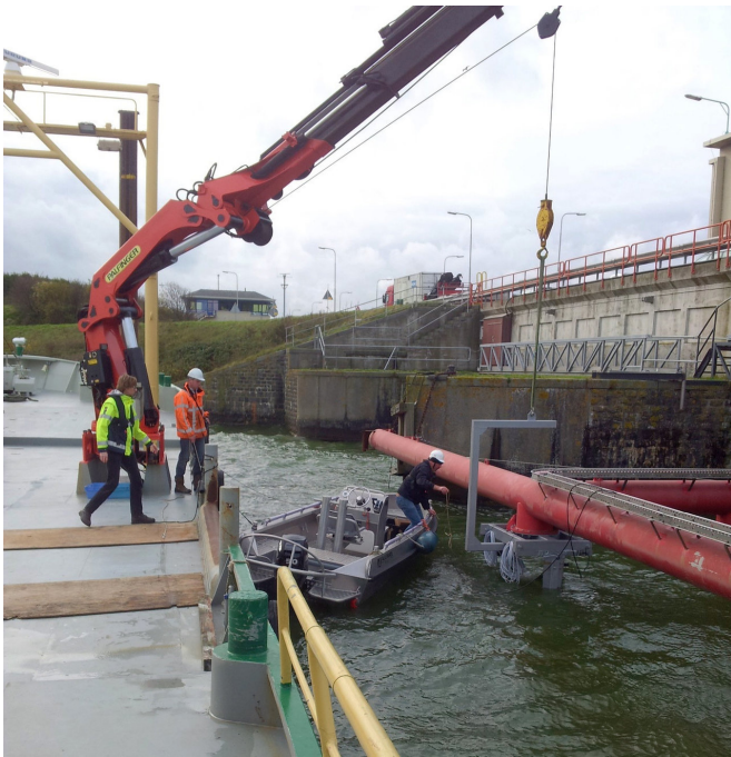
The hydrofoil's performance was tested using a custom-built instrumentation platform and mounting system. Credit: Trinity College Dublin
